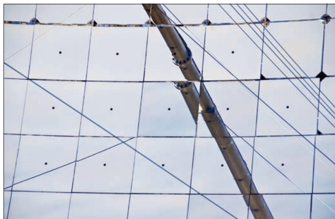
The “staggered” image in MAGIC-II demonstrates the action of the active mirror control. This normally operates on the individual mirrors to ensure the correct parabolic shape for the overall reflecting surface. The mirrors are mounted on three points, two controlled by actuators.
